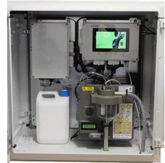
Photo showing the MS3500, Ammonia Monitor for Raw Wastewater
